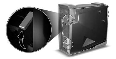
b Hold the rear edge of the panel with both hands then slide the panel towards the rear of the chassis.
